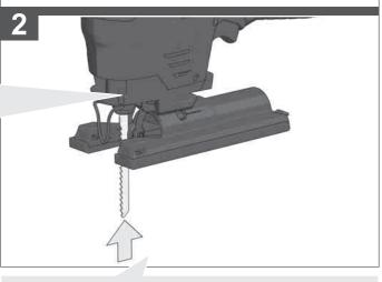
Press the saw blade into the Fixtec holder up to the stop.
