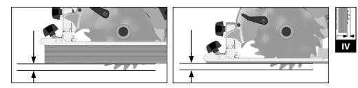
Adjust the cutting depth to the thickness of the workpiece. Less than a full tooth of the blade teeth should be visible below the workpiece.
