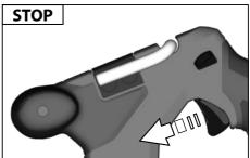
For safety reasons this power tool is fitted with a switch lock and the 0n-/0ff switch cannot be locked in the "0n" position.
