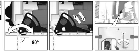
If a correction of the 90° angle of the guide-plate to the saw blade is necessary, use the correction screw.
