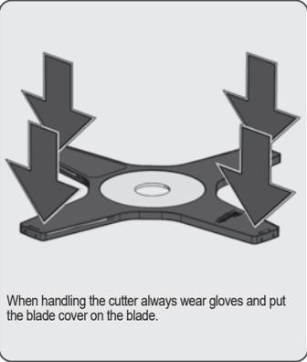
When handling the cutter always wear gloves and put the blade cover on the blade.
