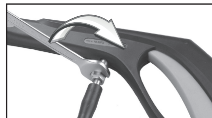
Installation of the pressure hose on model HPC 1800 Fig.8
