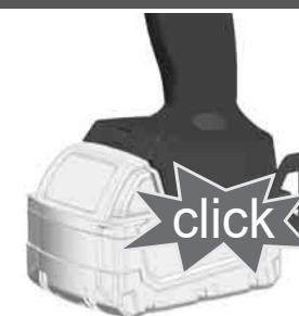
Remove the battery pack before starting any work on the machine.
