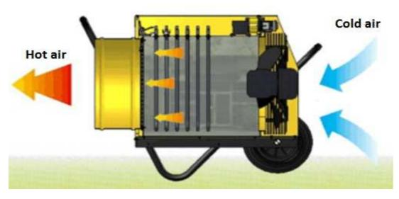
The device works on the principle of forced convection. The air flow is forced by a fan. Cold air is sucked from the back of the unit. The resistances heat the air. The heated air is expelled from the front of the heater. The unit is equipped with thermal protection with reset and a cooling thermostat. Switch positions: ventilation, heating with half power, heating at full power.
