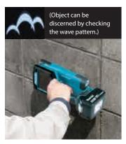
For detecting composite objects, such as rebars and cavities, in concrete block or brick wall
