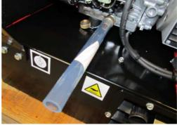
Mount the oil drain hose to drain the oil.
