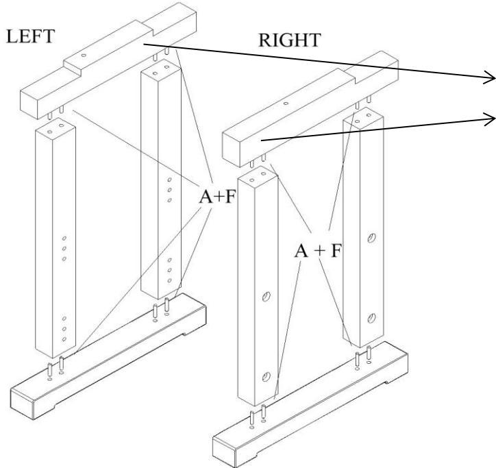
**ENG:** These parts are already mounted on the bottom of the workbench top. Please continue in assembly without these parts.
