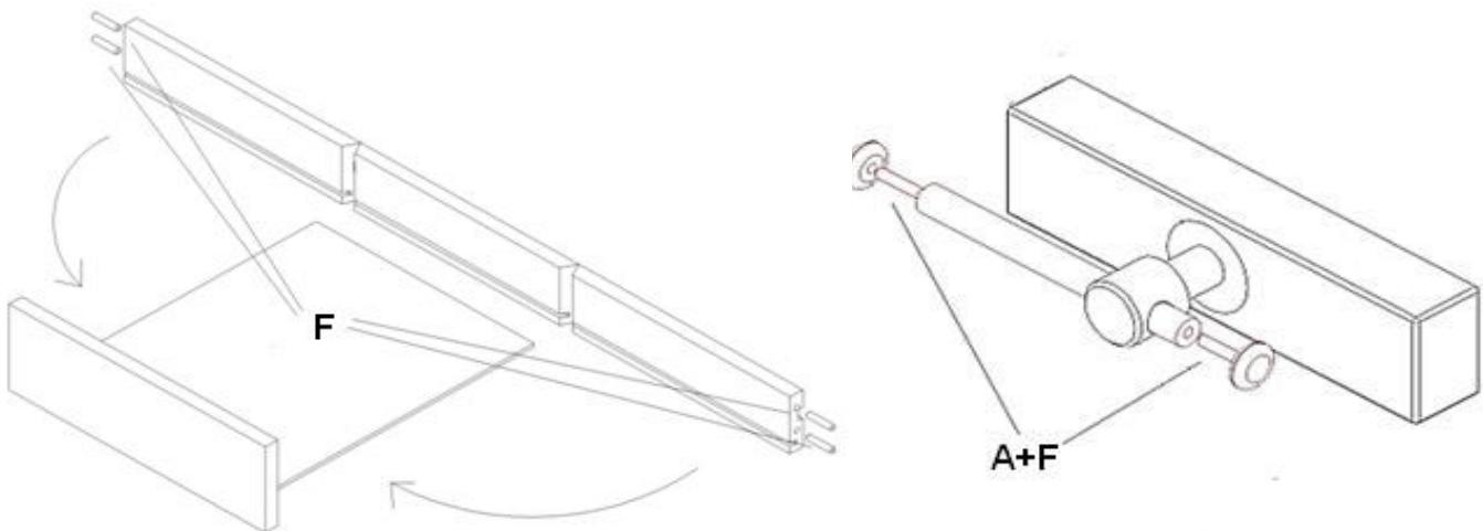
!!! HINT !!! - don't fill up holes for dowels by glue. Smear dowels by glue and insert them into holes.
