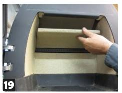
Let the plate rest on the rail with the air slots
