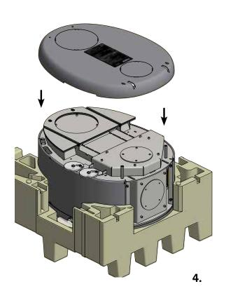
Mount the bottom plate on the existing four screws.
