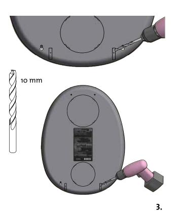
Mount the rear plate loosely; it is not to be fixed, until after the wall fitting has been mounted.
