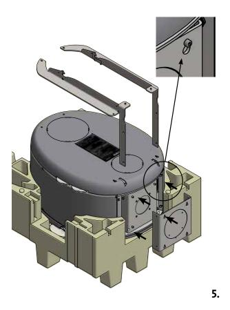
Let the rails glide down through the hole along the bottom plate.
