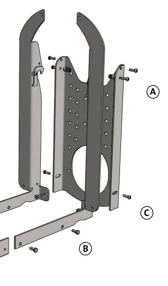
Mount the wall fitting on the wall. It is important that it is level. Mount bushing, screw and nut.
