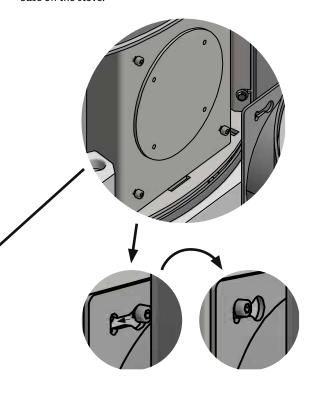
Place the delivered magnets on the markings on the front of the base and mount the loose front. Please note that the base can be mounted at the right or at the left of the stove.
