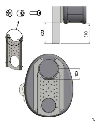
Dismount the rear plate by removing the four screws. Place the rear plate on an even surface.
