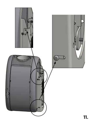
Replace the type plate on the stove with the one delivered with the wall fitting.
