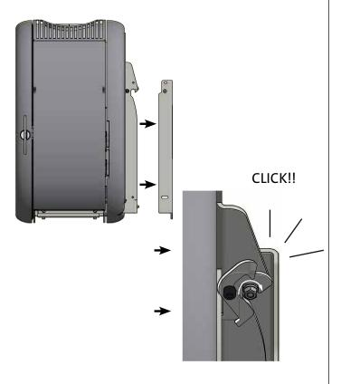
Adjust the stove to that the doors has the correct slope.
